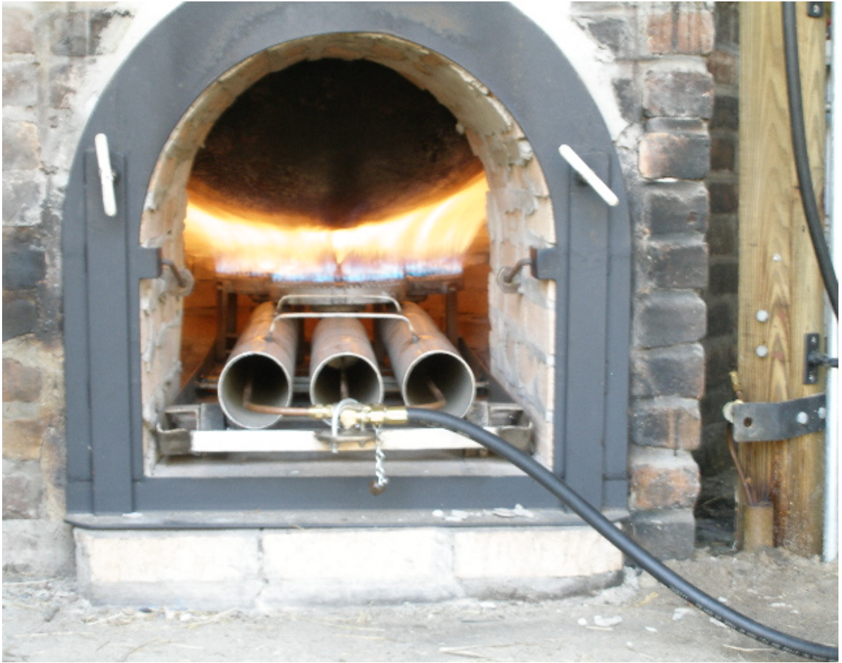
Syrup Kettle Burner (Firing at 10 psig) W. Olin Pope Farm, Barwick , Georgia
