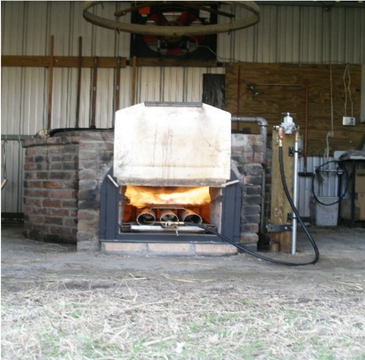
Syrup Kettle Burner (Firing at 20 psig) W. Olin Pope Farm, Barwick, Georgia
