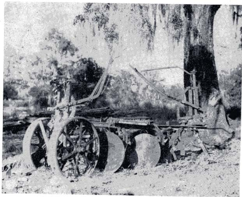
Photo No. 9. A very early Thomson Single Row Cane Plow.
