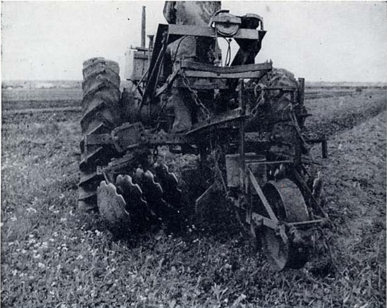
Photo No. 15. Corn planting implement attached to an Allis Chalmers UC Tractor.
