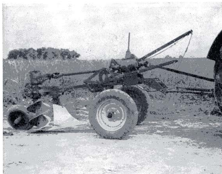
Photo No. 14. Parson's Whirlwind Terracing Plow.
