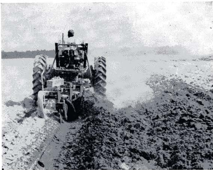
Photo No. 13. Thomson Disc Gang Plow.
