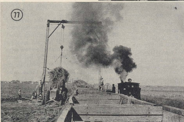
80. Sugar Mill—Unloading Cane Trucks and Tractors
