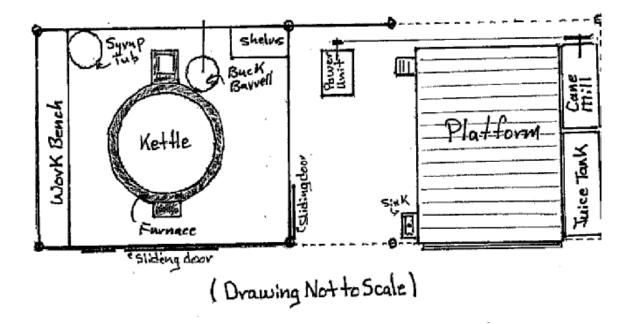
The syrup house is a wood frame and pole constructed building with the kettle totally enclosed. The cane juice is pumped underground from the holding tank to the kettle.
