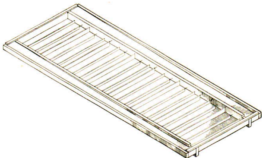
FIGURE 13.—Evaporator with skimming troughs.
