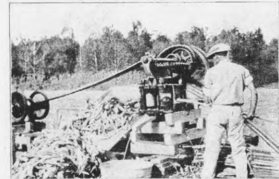
The belt-power attachment increases the capacity and efficiency of the mill.
