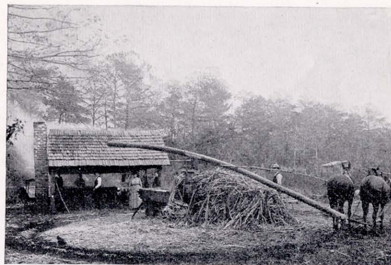
FIGURE 15.—Sirup-making outfit of type widely used by farmers who grow from 1 to 3 acres of cane. An outfit of this type has a capacity of 75 to 100 gallons of sirup per day and costs $150 to $200. The cost of larger capacity outfits equipped with power-driven cane mills is proportionately greater.
